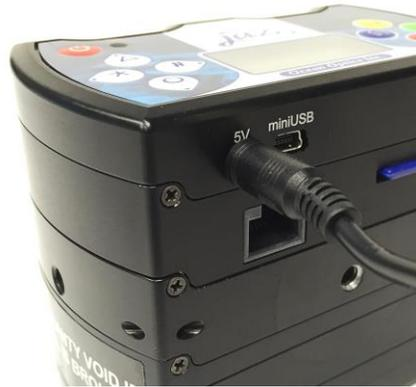
3. Now that the battery pack is connected to Jaz, you can monitor the charge state of the battery pack using the power Test button on the top of the battery pack as follows:
