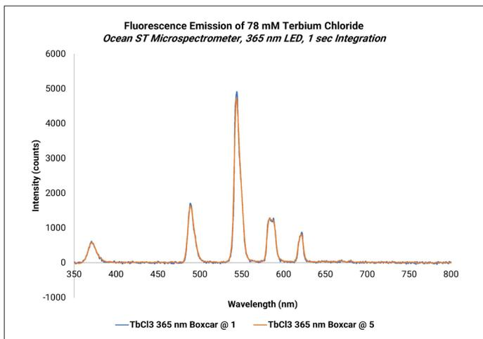
**Figure 2.** When excited with a 365 nm LED, the Terbium chloride solution revealed a strong fluorescence peak near 550 nm.
