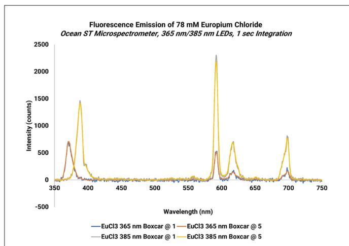
Figure 1. An Ocean ST microspectrometer measures the fluorescence response of Europium chloride. System flexibility allowed us to optimize excitation wavelengths and boxcar averaging.
