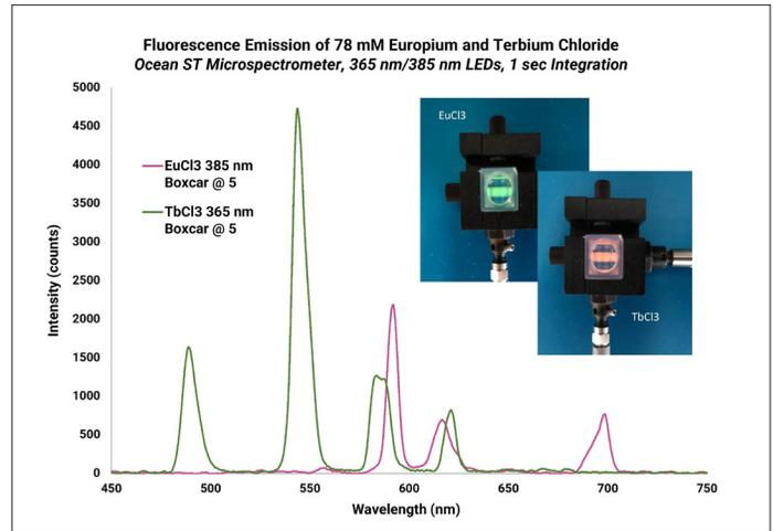
*Figure 3. Differences in Europium chloride and Terbium chloride fluorescence peaks correlate to the color of each compound's emissive glow.*
