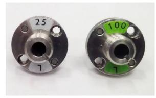
The slit size is indicated on the SMA connector for easy identification as shown here.
