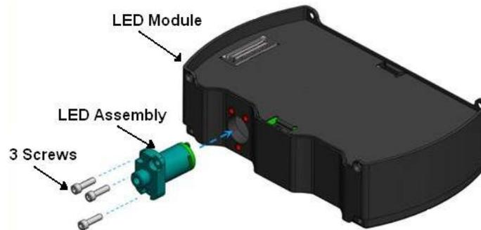
4. Completely remove the screws and set them aside for use in the new LED assembly.
