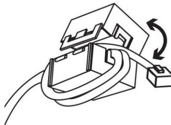
5. Snap the ferrite closed to lock it in place.
