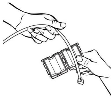
4. Loop the Ethernet cable through the ferrite twice.
