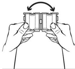
3. Place the ferrite on the Ethernet cable as close to the connector for the computer as possible.
