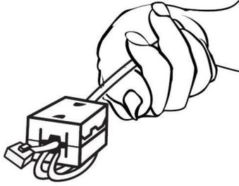
6. Plug the Ethernet cable into the Ethernet connector on the JAZ-E module, and then to a Power Over Ethernet (POE) bridge or switch to the network (e.g., an 8-port network hub).
