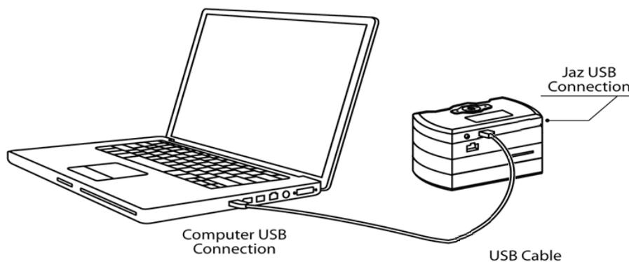
2. When first connecting Jaz to your computer, you must run the Hardware Wizard for your PC to recognize the new hardware. For Mac users, this step is not necessary.
