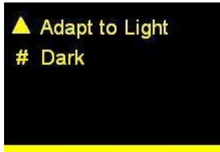
3. Take a dark measurement. To do this, cover the probe and press the # key for the Dark selection. Once Jaz has finished, the following screen appears:
