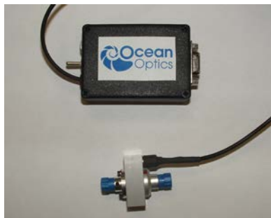
Inline TTL Shutter (bottom) with 15-pin input component and control circuitry (top)
