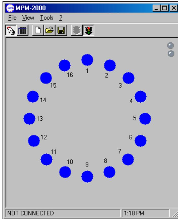
Channel Mode allows you to change the active channel on the MPM-2000. You can click on any of the blue buttons associated with the SMA 905 Connectors on the front of the MPM-2000 to activate that channel.
