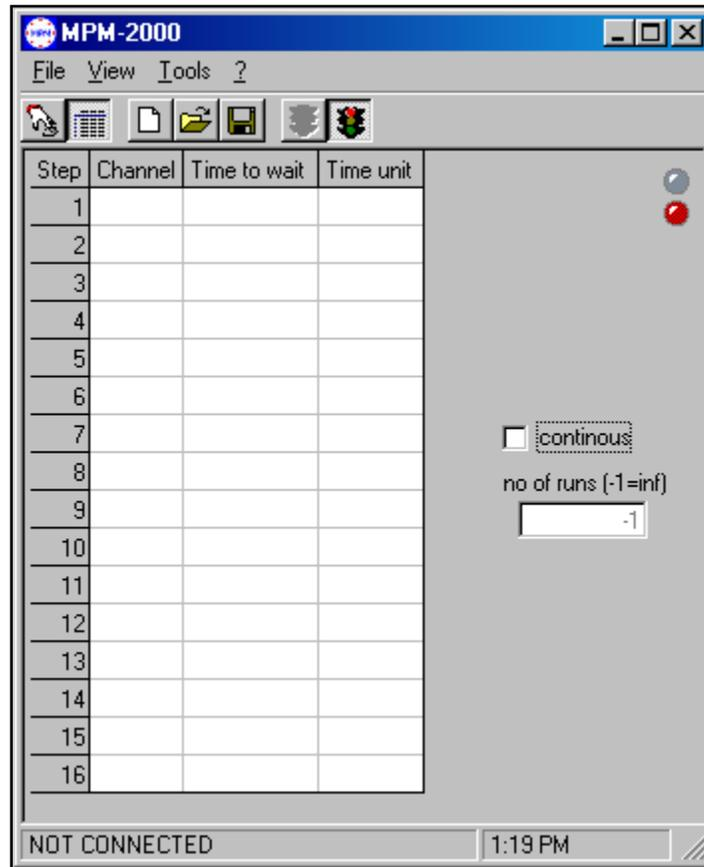
Program Mode allows you to create or change sequence programs used by the MPM-2000. The Program Mode interface contains the following items:
