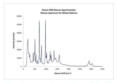
Xylene samples were measured using an Ocean HDX Raman with 25 µm slit for good resolution.
