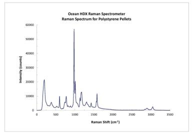
Ocean HDX Raman is a good option for measuring hydrocarbon polymers like polystyrene.
