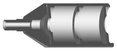
Gershun Tube – Cutaway view of product interior
