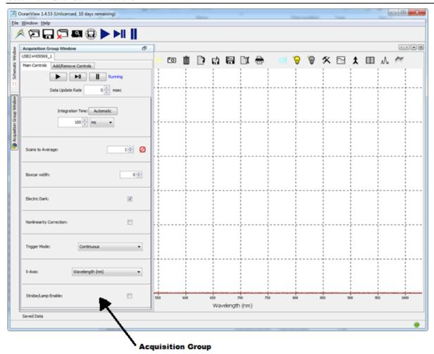
Different types of acquisitions are available for different devices. These devices include Spectrometer, I<sup>2</sup>C, SPI, Board Temperature, Thermo-Electric Cooling, and Analog In. The controls available in the Acquisition Parameters Controls vary based on the type of acquisition selected.
