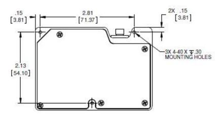
Figure 1: Flame Outer Dimensions
