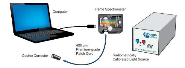
Typical Set-up for an Absolute Irradiance Measurement Using Field Calibration with a Calibrated Light Source
