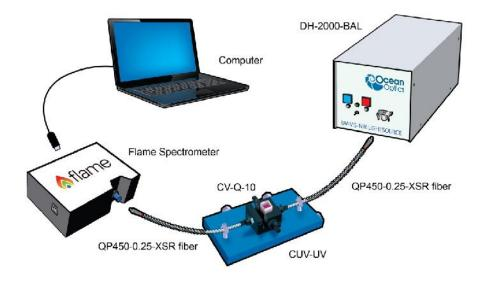
Ocean Optics Flame Fiber Optic Spectrometer Typical Set-up
