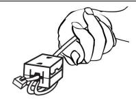
6. Plug the Ethernet cable into the Ethernet connector on the JAZ-E module, and then to a Power Over Ethernet (POE) bridge or switch to the network (e.g., an 8-port network hub).
