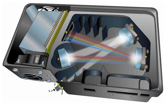
**QE65 Pro Spectrometer with Components**
