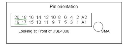
22-Pin Accessory Connector Pinout Diagram
