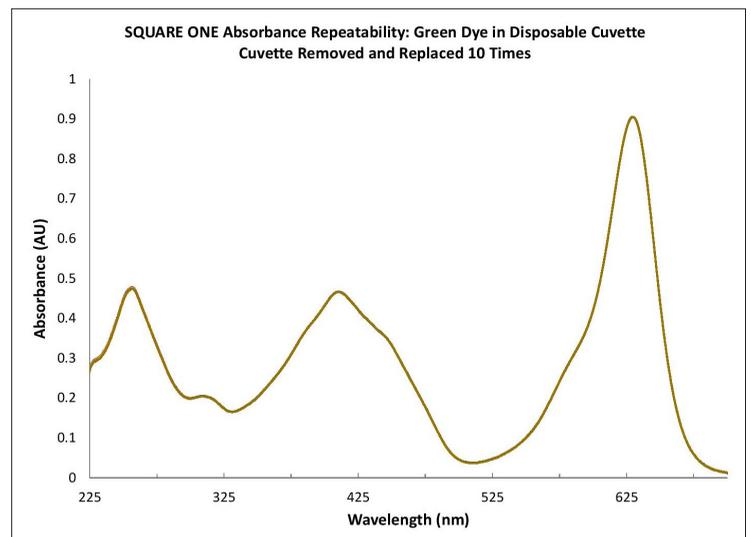
*SQUARE ONE spectral repeatability when a disposable cuvette containing a concentrated green food dye is removed and replaced in the cuvette holder 10 times. Even with disposable cuvettes, the spectra overlay almost perfectly, with an average absorbance of 0.47 AU at 410 nm with standard deviation of just 0.0008 AU.*
