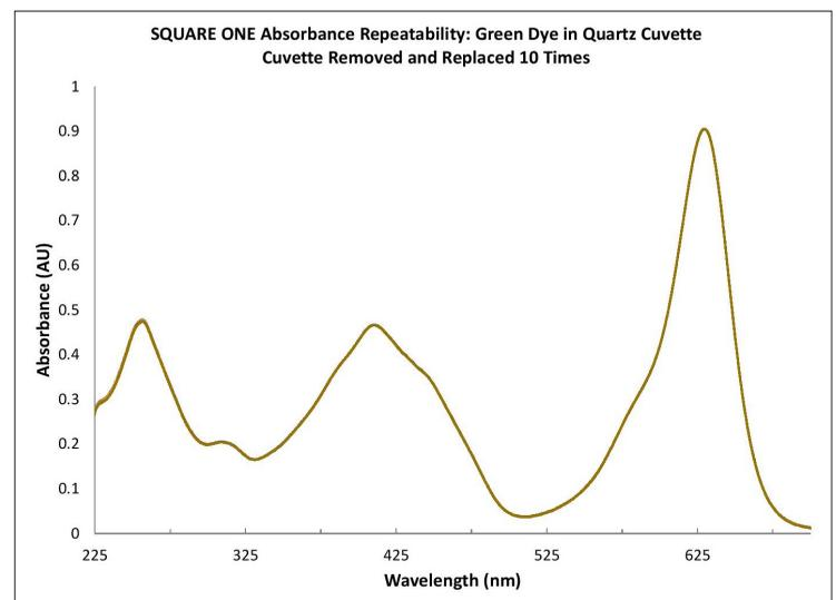
*SQUARE ONE spectral repeatability when a quartz cuvette containing diluted green food dye is removed and replaced in the cuvette holder 10 times. The spectra overlay almost perfectly, with an average absorbance of 0.47 AU at 410 nm with standard deviation of just 0.0007 AU.*
